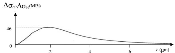
**Figure 6.** Radial profile of stress birefringence ( $\sigma_{rr} - \sigma_{\theta\theta}$ ).
