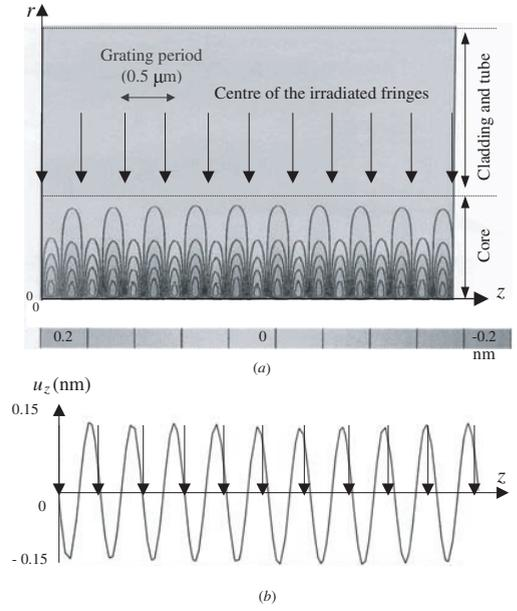
**Figure 4.** (a) Axial displacement distribution in the fibre section. (b) Axial profile at  $r = R_c/4$ .
