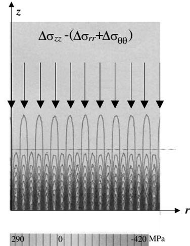
**Figure 9.** Test of the sum rule  $\sigma_{zz} = \sigma_{rr} + \sigma_{\theta\theta}$  in a fibre section containing a Bragg grating.
