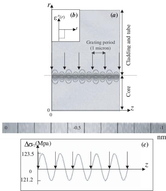
**Figure 8.** (a) Shear stress  $\Delta\sigma_{rz}$  for a step densification profile shown in (b) and a grating period of  $1\mu\text{m}$ , (c) is the axial profile at the core-cladding interface, i.e.,  $\Delta\sigma_{rz}(r = R_c)$ . The black arrows along the grating in (a) and the black arrows in (c) indicate the centre of the irradiated fringes.
