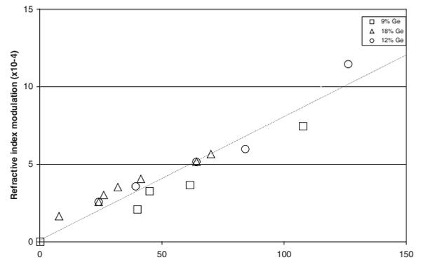
**Figure 10.** Relationship between refractive index modulation and the mean axial stress change for three different fibres (after [15]).
