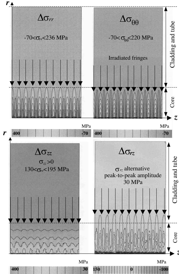
**Figure 5.** The three diagonal ( $rr$ ,  $\theta\theta$ ,  $zz$ ) and the shear ( $rz$ ) components of the stress tensor in MPa. The black arrows along the grating indicate the centre of the bright fringes.
