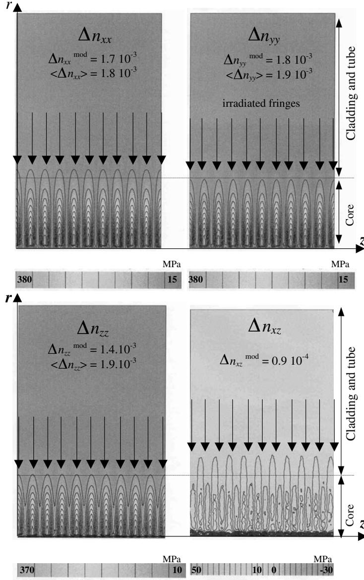
**Figure 7.** The three diagonal ( $xx$ ,  $yy$ ,  $zz$ ) and the shear ( $xz$ ) components of the refractive index change tensor in a Cartesian coordinate system ( $\theta = 0$ ). The black arrows along the grating indicate the centre of the irradiated fringes.
