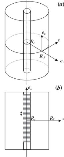
**Figure 1.** Optical fibre structure in the cylindrical coordinates system: (a) Three-dimensional scheme of the fibre showing the inner cylinder representing the core region of radius  $R_c$  and the outer cylinder of radius  $R_f$ . (b) Two-dimensional scheme of the longitudinal fibre section containing a Bragg grating of pitch  $\Lambda$ .
