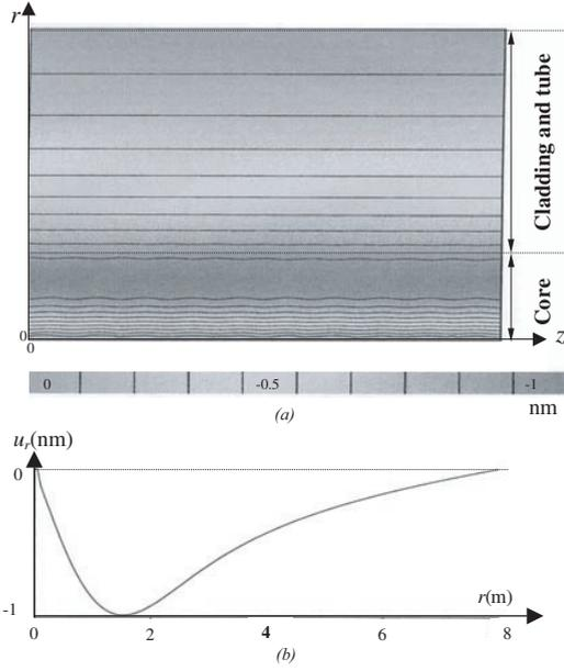
**Figure 3.** (a) Radial displacement distribution in the fibre section. (b) Radial profile at  $z = 0$ .
