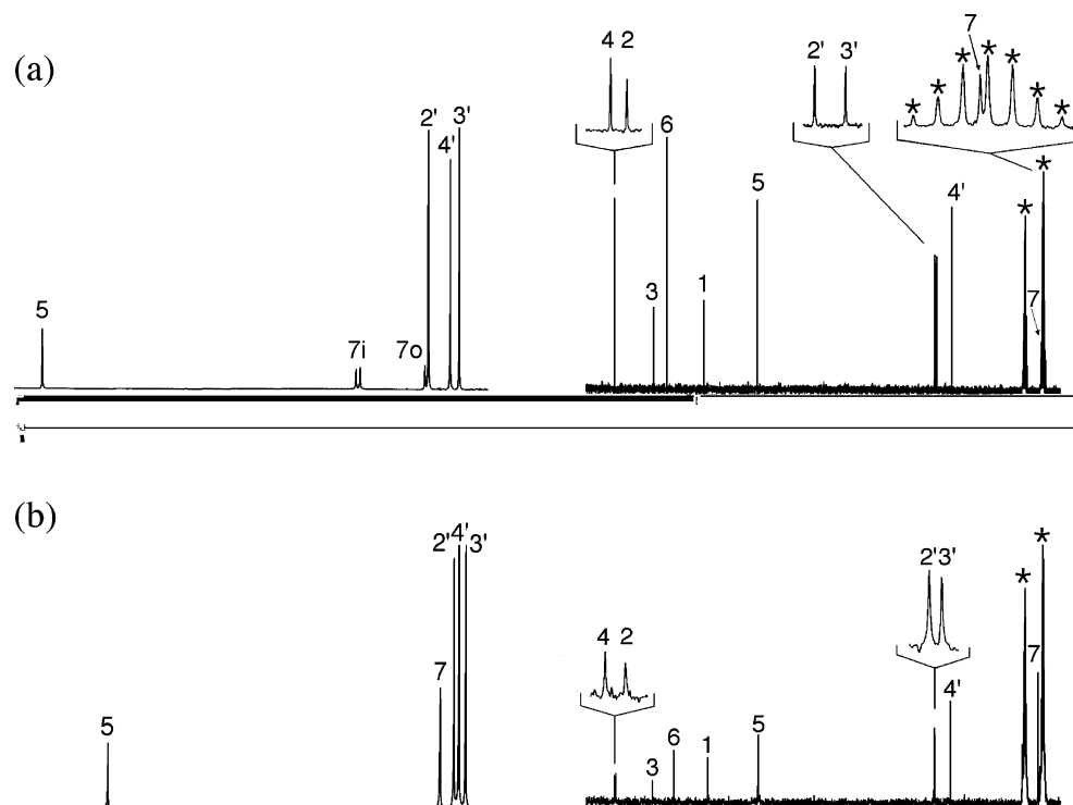
Figure 2. 400.1 MHz ^1\text{H} (left) and 100.6 MHz ^{13}\text{C}-\{^1\text{H}\} (right) NMR spectra of the (a) crown and (b) saddle isomers of 1 dissolved in \text{DMF-}d_7 at room temperature. Expanded regions are shown for closely spaced peaks in the ^{13}\text{C} spectra. Peaks labeled with asterisks correspond to \text{DMF-}d_7 .
