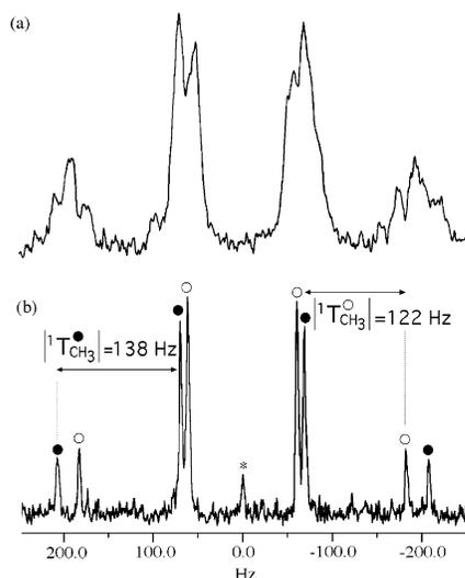
**Figure 6.** Signal of the methyl group of (*rac*)-7 extracted from the <sup>1</sup>H-coupled <sup>13</sup>C spectrum (a) and <sup>13</sup>C-<sup>1</sup>H HETSERF 2D map (b). The 1D spectrum was recorded with 2000 scans. In both cases, a Lorentzian filtering was applied (LB<sub>1,2</sub> = 2 Hz). The small peak at 0 Hz is an artifact.
