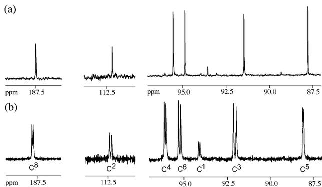
**Figure 4.** Part of the deshielded region of the 100 MHz  $^{13}\text{C}\{^1\text{H}\}$  NMR spectrum of *rac*-**1** dissolved in (a) chloroform and (b) PBLG/chloroform. Both spectra were recorded with 4000 scans. Exponential (LB = 1 Hz) and Gaussian filtering (LB = -2 Hz, GB = 70%) were applied, respectively.
