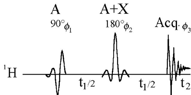
Fig. 1. Basic pulse scheme of the SERF 2D experiment. The first selective-excitation  $90^\circ$  pulse uses an EBURP-2 shaped pulse while the doubly selective  $180^\circ$  pulse uses the REBURP shaped pulse. The 4-steps phase cycling of the SERF sequence used was  $\phi_1 = \phi_{\text{acq.}} = x, -x, -x, x$  and  $\phi_2 = x, x, x, x$ .
