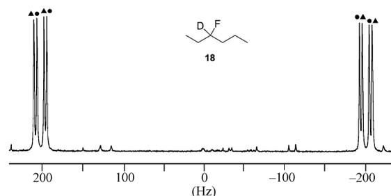
**Fig. 1** <sup>2</sup>H-{<sup>1</sup>H} NMR spectrum of 3-deutero-3-fluorohexane **18** in a solution of PBLG–CHCl<sub>3</sub> (13 wt% PBLG) at  $T = 302$  K. Peaks marked with ● belong to one enantiomer and those marked with ▲ are due to the other enantiomer.
