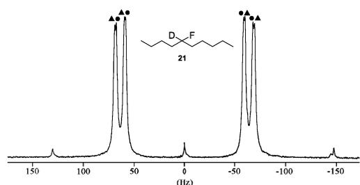
**Fig. 2**  $^2\text{H}\{-^1\text{H}\}$  NMR spectrum of 5-deutero-5-fluorodecane **21** in a solution of PCBL–DMF (27 wt% PCBL) at T = 320 K. Peaks marked with ● belong to one enantiomer and those marked with ▲ are due to the other enantiomer.
