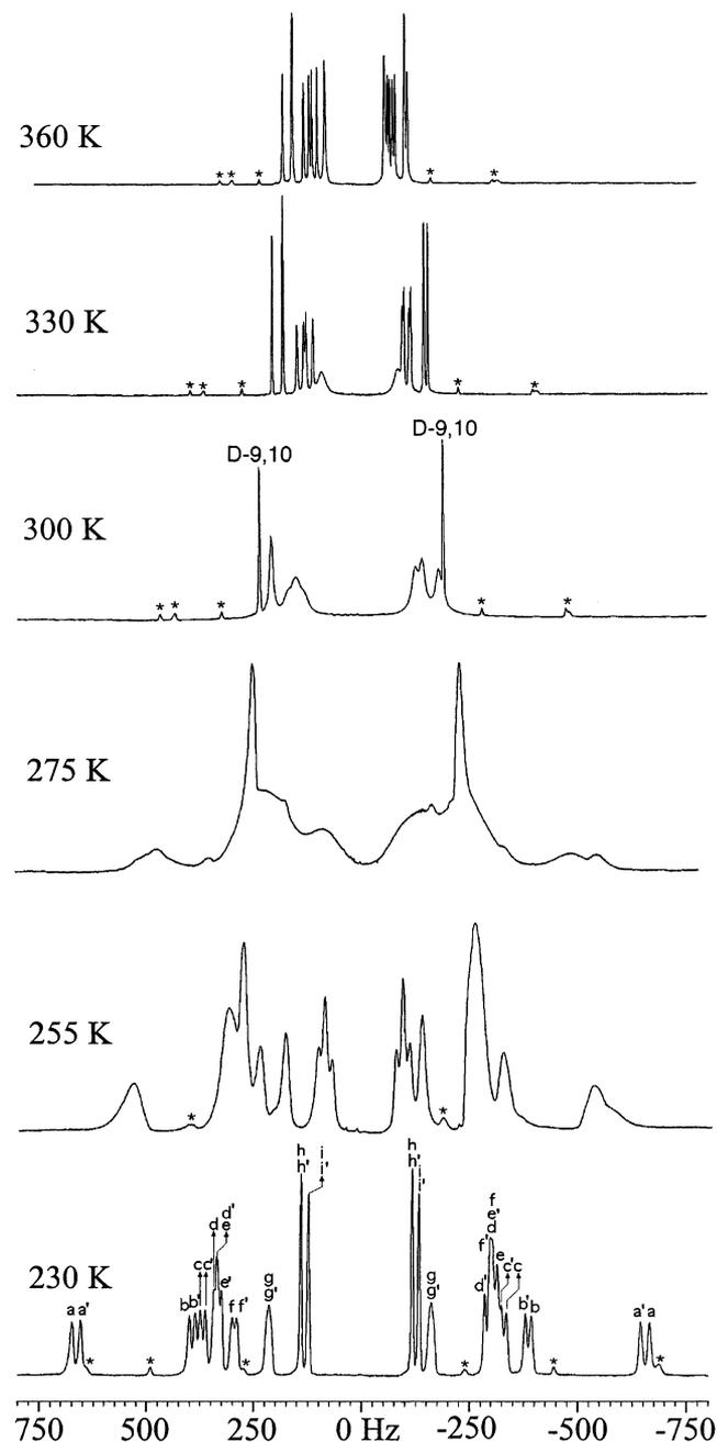
**Figure 3.** 61.4 MHz deuterium NMR spectra for  $1\text{-D}_{18}$  in PBLG/ $\text{CHCl}_3$  phase as a function of temperature. 208 scans of 3 k data points were added for each spectrum and a recycle delay of 1.5 s was used. Gaussian filtering and zero filling to 16 k data points were employed to improve the spectral appearance and the digital resolution.
