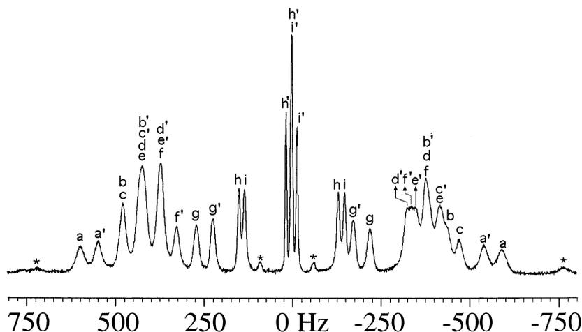
**Figure 5.** 61.4 MHz deuterium 1D spectrum for **1-D**<sub>18</sub> at 240 K in the PCBL/ $\text{CH}_2\text{Cl}_2$  phase. 208 free induction decays were added. No filtering was used.
