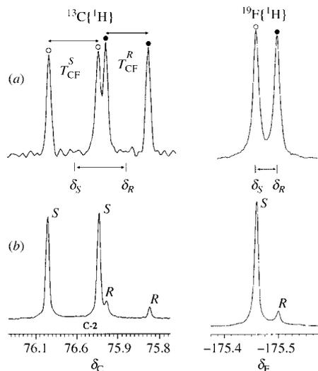
**Fig. 2** <sup>19</sup>F{<sup>1</sup>H} spectrum and <sup>13</sup>C{<sup>1</sup>H} NMR signal associated to the C-2 carbon of (a) (±)-**2b** and (b) (–)-**2b** recorded at 294 K by adding 64 and 1500 scans, respectively. Gaussian filtering was applied to enhance the spectral appearance. For (±)-**2b**, we measure  $T_{CF}^S = \pm 12.8$  Hz,  $T_{CF}^R = \pm 11.1$  Hz for the C-2 carbon.
