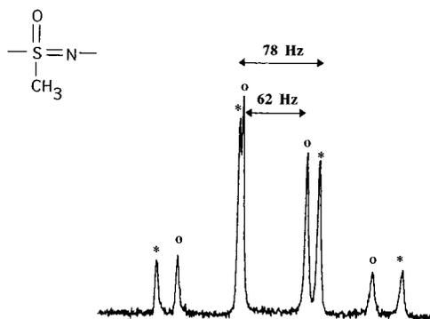
**Figure 6.** Doubled quartet associated to the methyl (C6) group of *S*-methyl-*S*-*P*-tolyl-*N*-tosylsulfoximine observed on the proton decoupled carbon-13 spectrum at 300 K. Fifteen hundred scans were collected. The peaks due to each enantiomer are labeled by (o) and (\*). The decoupling was applied during the relaxation delay period to gain the Nuclear Overhauser Effect.
