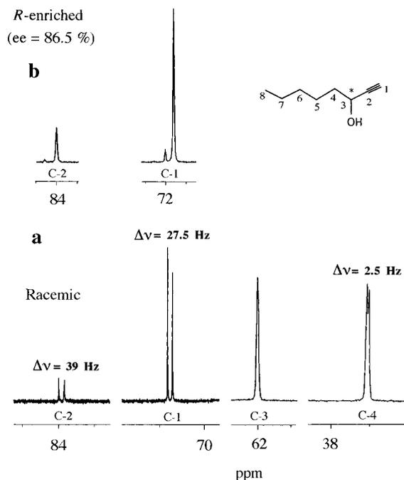
**Figure 2.** (a) Expansion of the <sup>13</sup>C-<sup>1</sup>H spectrum of (±)-oct-1-yn-3-ol (54/100/555/14.1%) dissolved in PBLG/CDCl<sub>3</sub> at 300 K. Two thousand scans were added. Note the large Δν differences on the sp carbons. (b) <sup>13</sup>C-<sup>1</sup>H spectrum of C-1 and C-2 of an R-enriched sample (87.3% ee) (59.9/80/521/12.1%). The spectrum was recorded with 5000 scans and 16 k of data points. The recycle delay was 2 s. The measured ee through integration was 86%.
