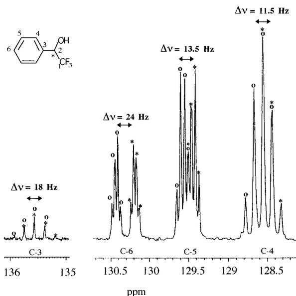
**Figure 7.** <sup>13</sup>C-<sup>1</sup>H spectrum of (±)-1-deutero-1-phenyl-2,2,2-trifluoroethanol (65/100/406/17.5%) dissolved in PBLG/CD<sub>2</sub>Cl<sub>2</sub> at 300 K. Twenty-two scans were added. The peaks due to each enantiomer are labeled by (o) and (\*), but the attribution for each carbon is arbitrary.
